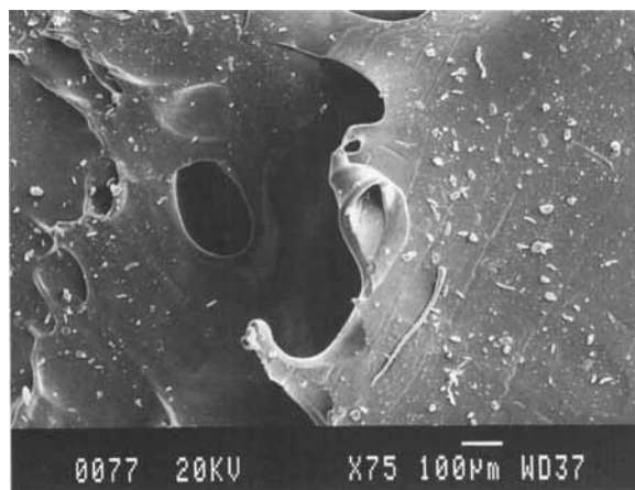
Figure 10 Scanning electron micrograph of peeled surface of rubber, in a system modified with block copolymer 4.
